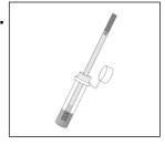
Insert a test strip into the solution and incubate at room temperature for **5 minutes**. **Read the result immediately**.
