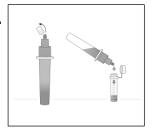
Remove the smaller cap to open the dropper tip, and transfer **6 drops** or **200 µL** into an incubation vial and close the lid.
